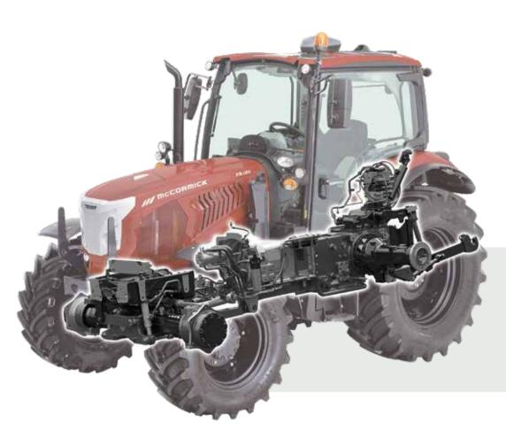
The **X5** features an open-centre hydraulic system with either a dual pump that provides a flow rate of 62 l/min or a triple pump with up to 82 l/min to operate the remote valves, the front and rear hitches and the front loader. A second pump with a flow rate of 32 l/min is dedicated to the steering system. This high hydraulic capacity allows the operator to:
